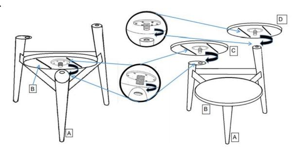
Place the table base (A) on a flat surface. Align threaded stud of Large Top (B) on shortest leg of the Table Base as shown above in drawing. Rotate Large Top (B) in clockwise direction until secured. Align Medium Top (C) on medium leg of the Table Base (A) and secure by rotating in clockwise direction. Align Small Top (D) on tallest leg of the Table Base (A) and secure by rotating in clockwise direction until secured. Do not over tighten all three Tops (B, C & D) on the Table Base (A).
